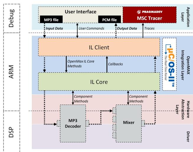
On our implementation, the different components (MP3 decoder, Mixer, Etc..) are running on an ARM core, but the processing in itself is entirely performed by a dedicated DSP.
