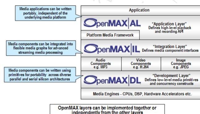
The OpenMAX IL API strives to give media components portability across an array of platforms. Each module is encapsulated in a component interface. OpenMAX defines three main types of entities:
